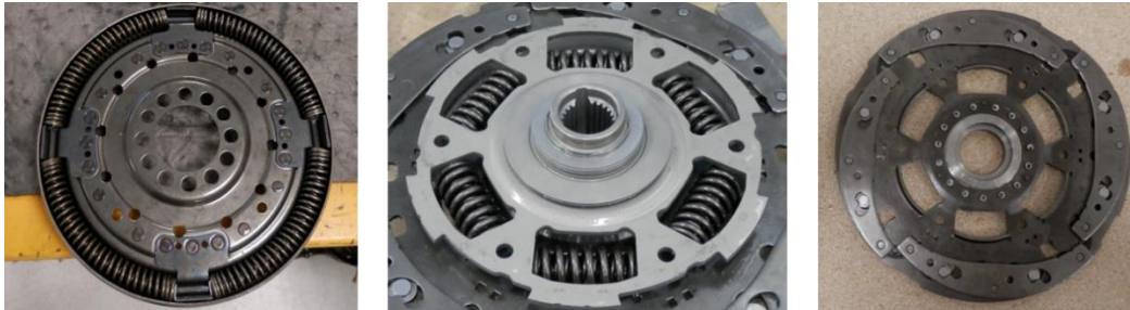
Figure 2 - CPVA assembled in the torque converter
